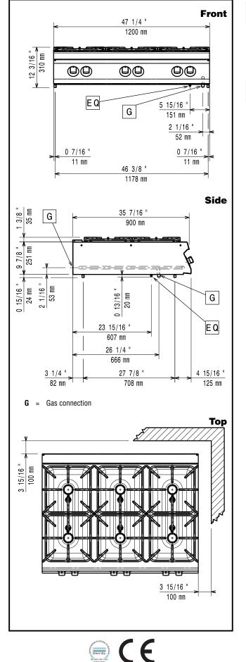
Modular Cooking Range Line EVO900 6-Burner Gas Boiling Top, 7.5kW - Town Gas
