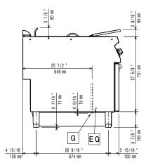
EQ = Equipotential screwG = Gas connection
