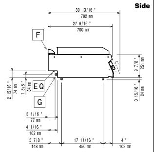
EQ = Equipotential screwG = Gas connection
